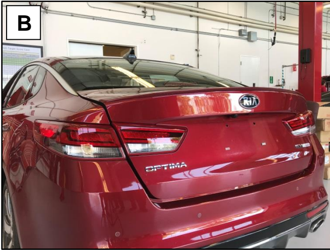
Trunk opening height not as designed.
