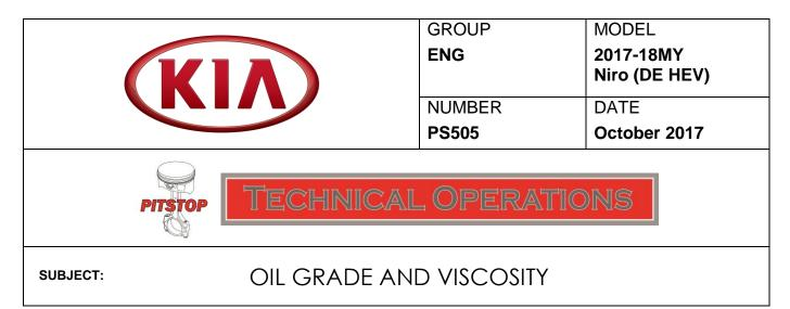
For 2017-18MY Niro (DE HEV) vehicles equipped with the 1.6L GDI Kappa engine, the recommended oil grade/spec to use is 0W-20 API SN synthetic oil or ACEA C2 SAE 5W-30 (petroleum based oil).
