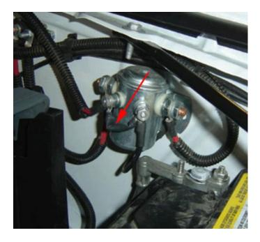
Important: Be sure to insulate the diode with heat shrink tubing before installing as shown in the picture above.
