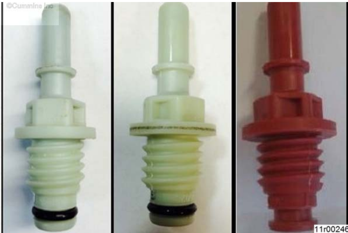
Figure 1, Revised Backflow Connector, Part Number 4387302, Installed in the Aftertreatment DEF Dosing Unit
