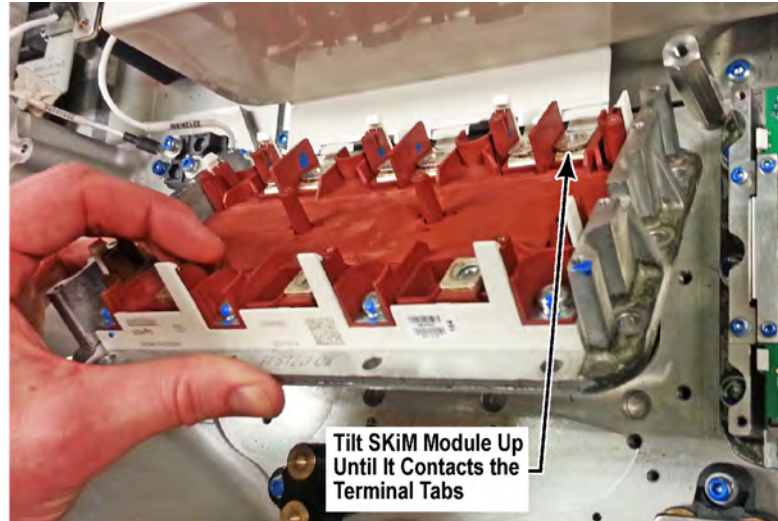
Figure 41. SKiM® Module Removal
