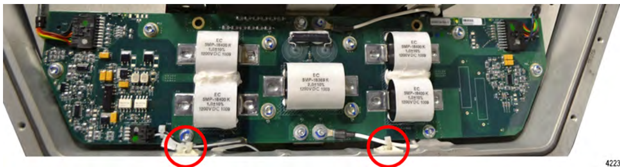
Figure 83. HVIL Circuit Card – Two (2) Wire Tie Locations
