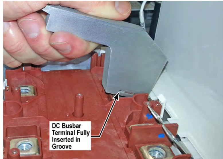
Figure 38. Inserting J-51586 Over DC Busbar Terminal Tab
