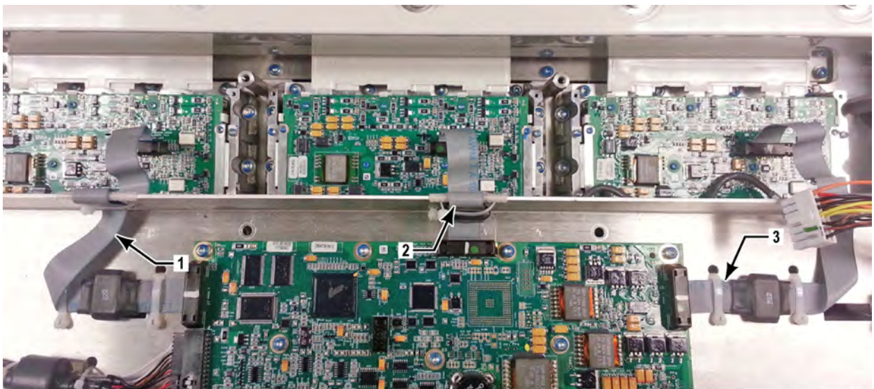
Figure 72. BCA Mounting Shelf (GATE Drive Card Cable Connectors Shown Circled)
