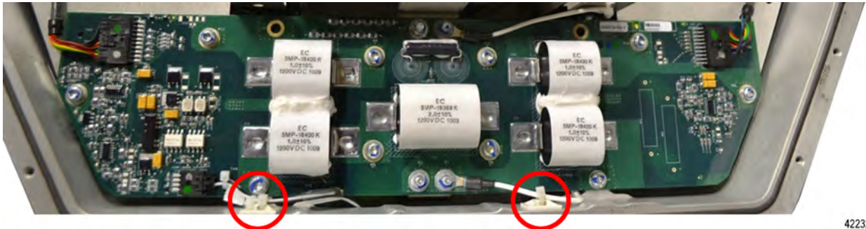
Figure 5. HVIL Circuit Card – Two (2) Wire Tie Locations
