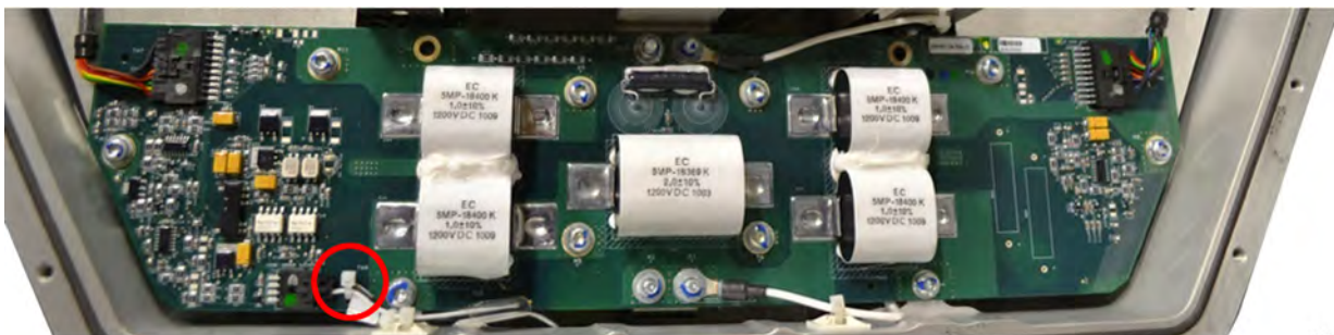
Figure 4. HVIL Circuit Card – Wire Tie Location
