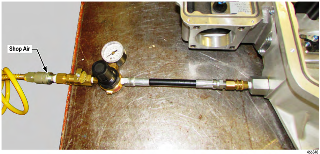
Figure 36. Connecting DPIM Leak Tester J-51673
