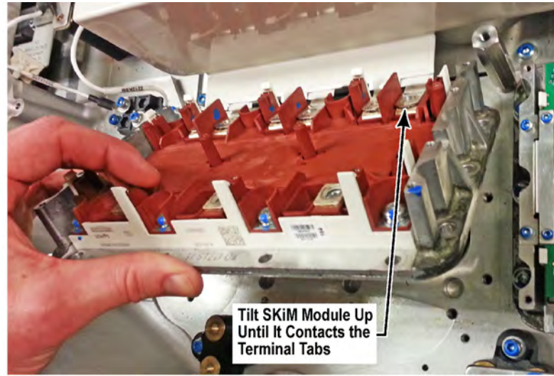
Figure 46. SKiM® Module Installation
