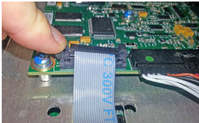
Figure 19. Releasing the Ribbon Cable Connector (BCA Cable Card Connector Shown for Clarity)
