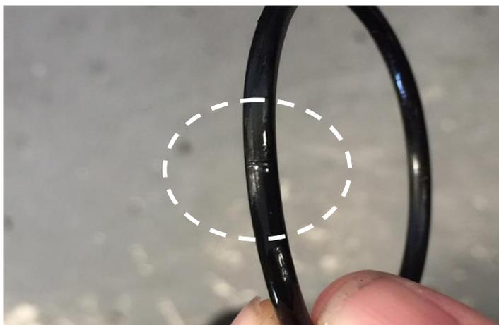
Replace the O-ring seal as necessary. Clean the Camshaft Adjustment Valve 1 -**N205**- and its connector of residual oil.
