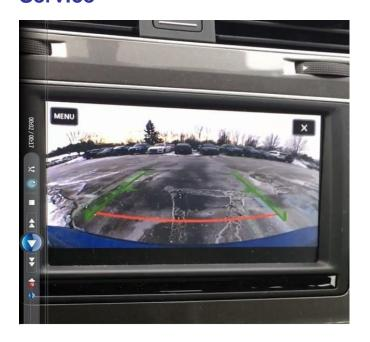
Place the vehicle in reverse with your foot on the brake to allow the rearview camera to activate.
