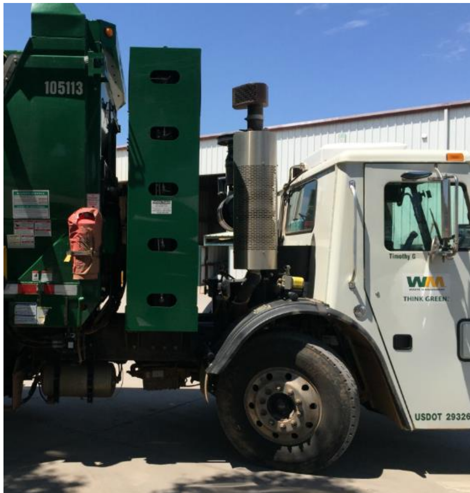
Figure 1. Behind the cab system number 22523000 mounted on a Mack LEU633 chassis.
