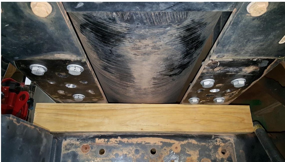
Figure 3. A piece of lumber (4 x 4 pictured) can be used to safely rest the fuel system on but above the vehicle chassis.
