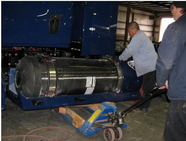
Figure 6. Use a jack or forklift to lift and pull the system from the mounting brackets.
