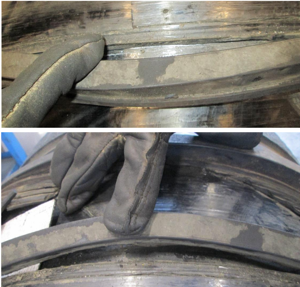
Figure 12. Isolator ribs that are damaged or de-laminated can be patched with a section of isolator material, part number 20100149.
