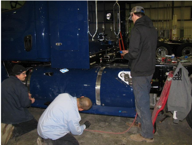
Figure 5. Remove the outer cover bolts and remove the top and side covers.
