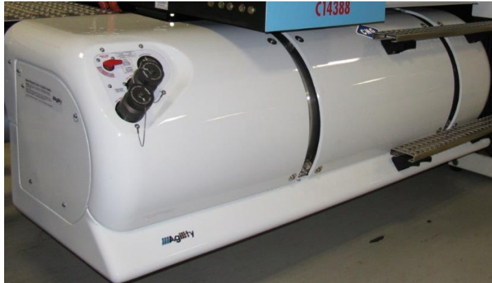
Figure 1. Side mounted CNG fuel system (237 series, Gen 3) affected by this procedure.
