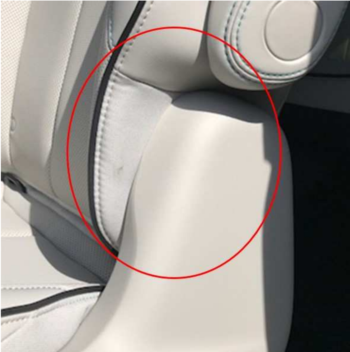
Fig. 6 Inspect for Grease
