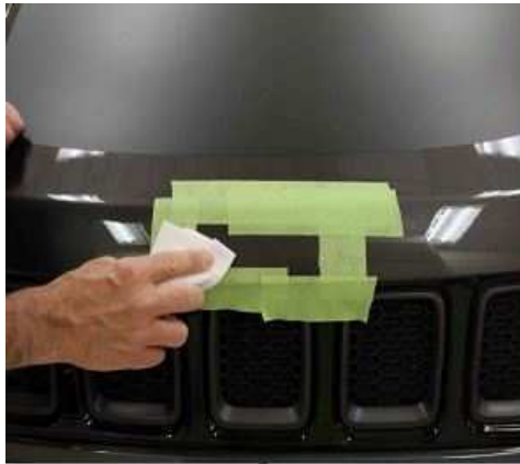
Fig. 5 Cleaning The Area
