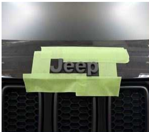
Fig. 6 Apply Nameplate With Firm Pressure
