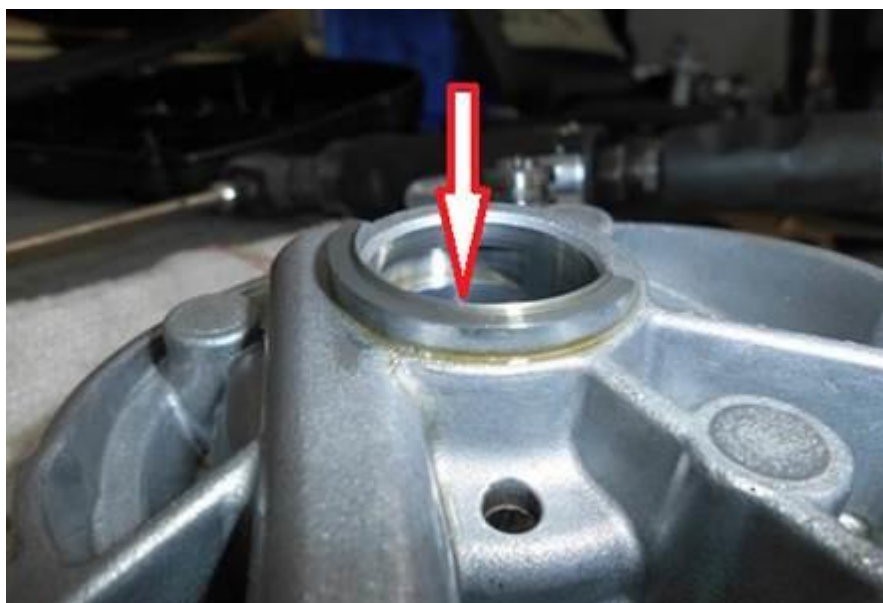
Figure 1) example of worn camshaft bearing bridge
