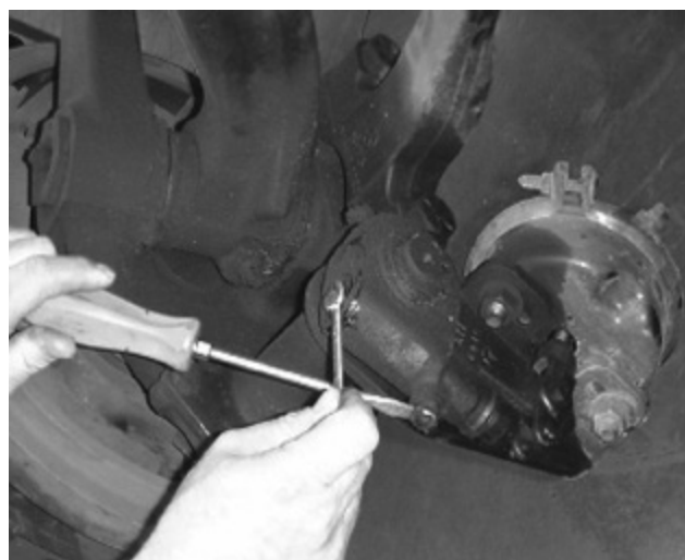
Figure 3: Retracting brake shoes
