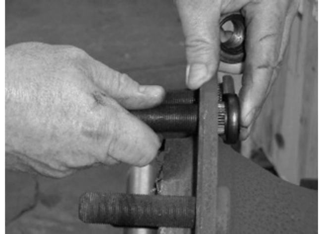
Figure 5: Installing new studs
