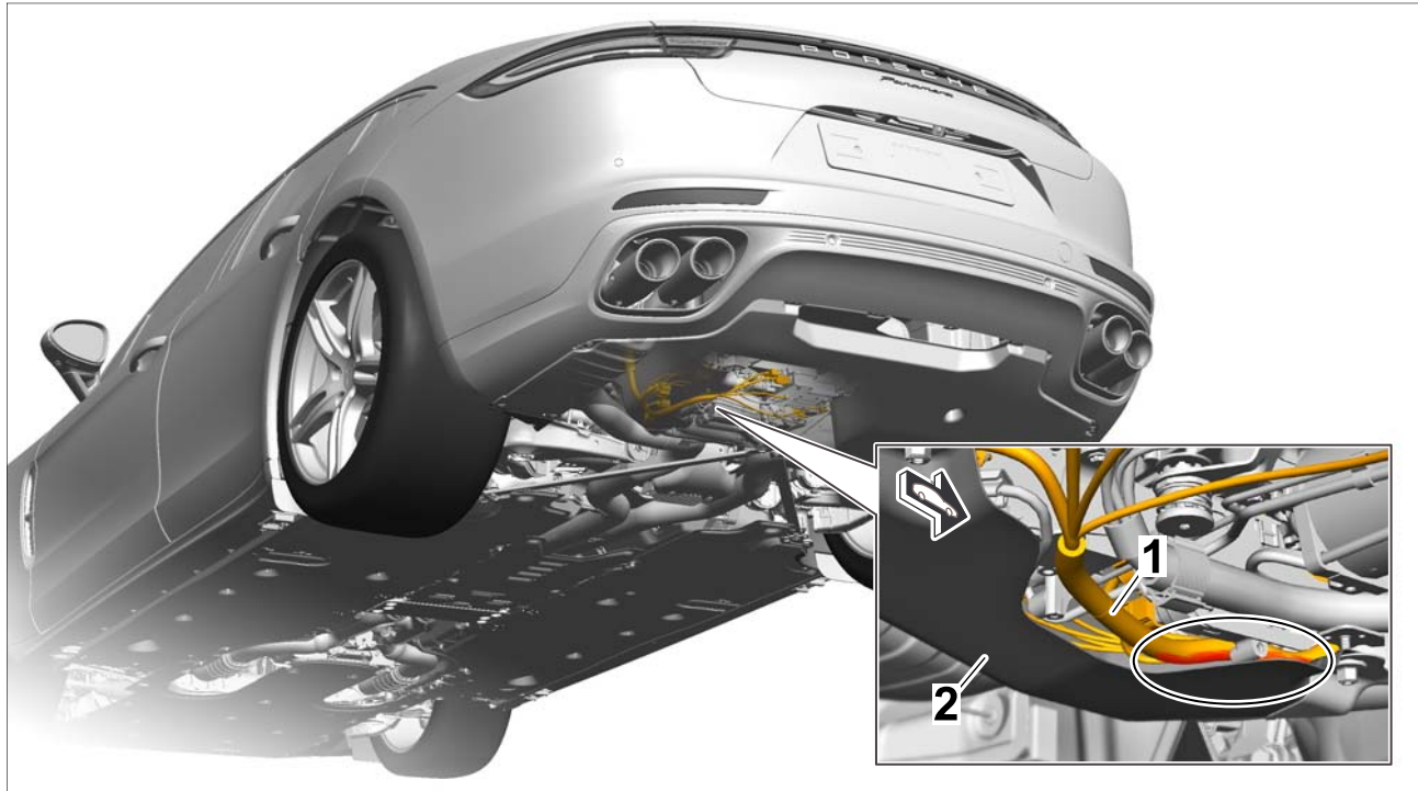
Installation position of wire harness for valve unit
