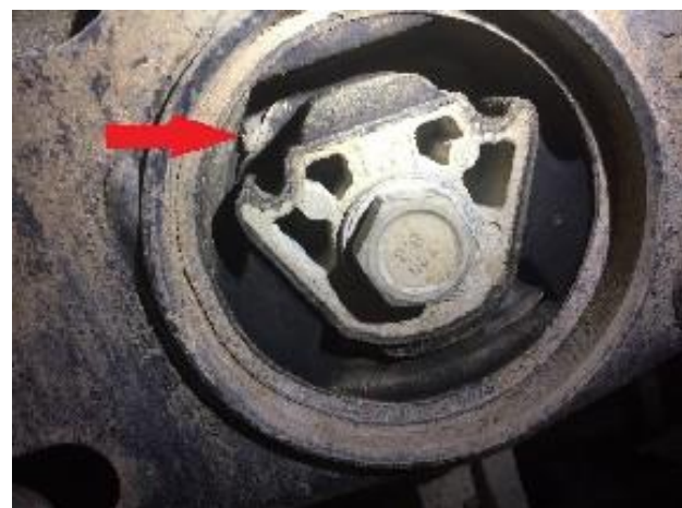
2. Stone trapped between inner and outer sections of the mount, causing bind
