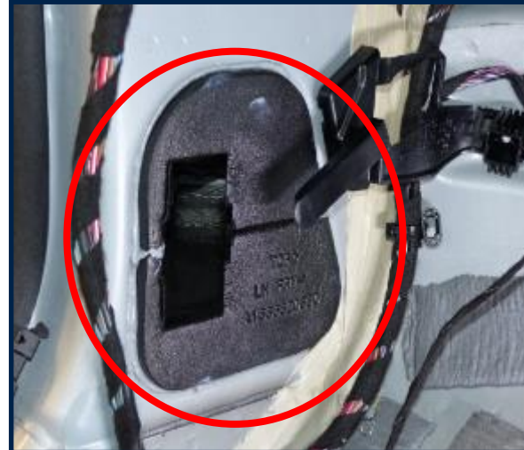
Bodyshell holes sealed
