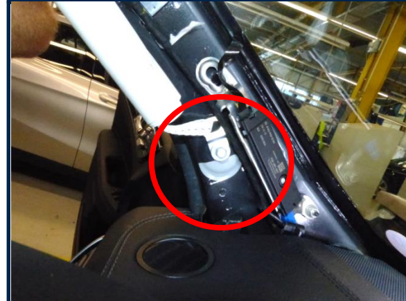
Bodyshell holes sealed
