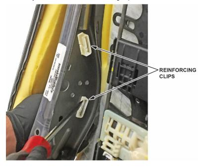
5. Install the counter-measure front seat side airbag holder.
