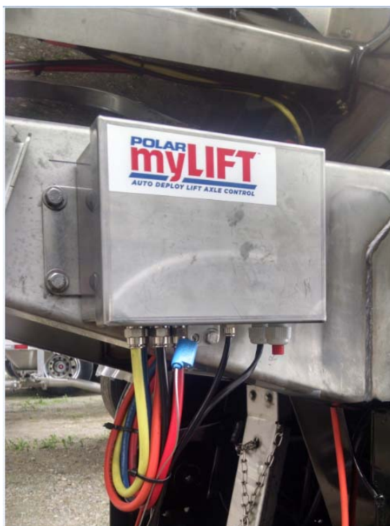
Picture 1 – MyLift control box is installed on the framing near the axles.
