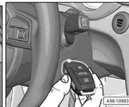
Figure 2. Hold top of key against coil.
