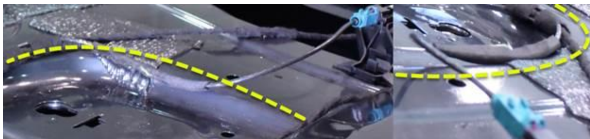
Figure 7. The coaxial line will run along the sheet metal stamp indent, as shown by the dashed line.
