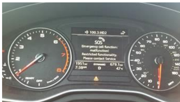
Figure 1. SOS warning in instrument cluster.
