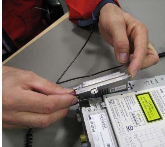
Figure 11. Remove the top out first.
