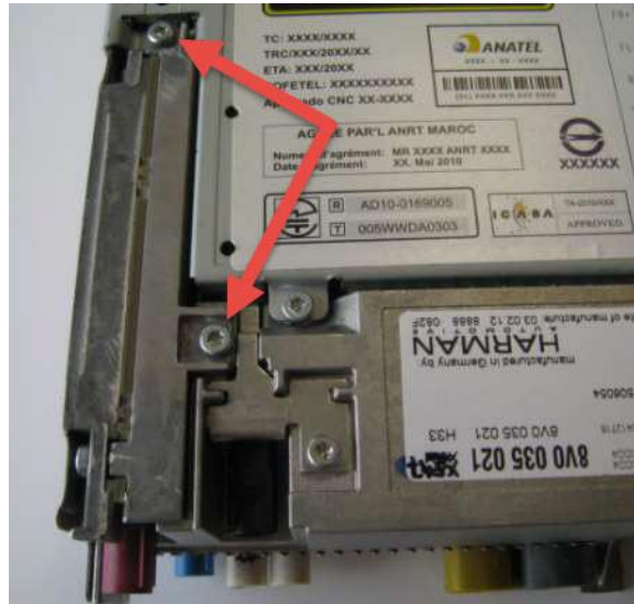
Figure 13. Do not over torque screws.
