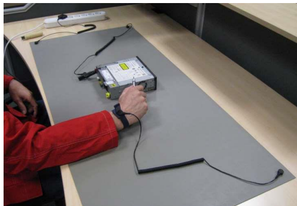
Figure 6. ESD Complete Setup.
