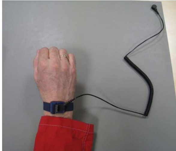
Figure 5. Human Ground Strap.
