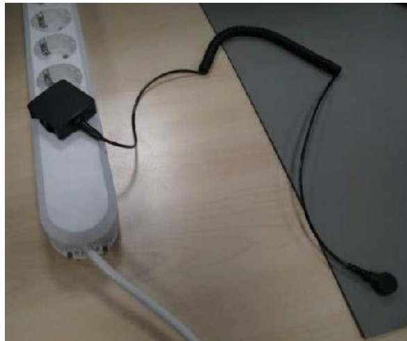
Figure 4. Grounded ESD Work Surface.
