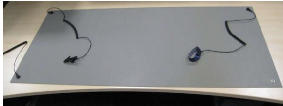
Figure 3. ESD Work Surface.
