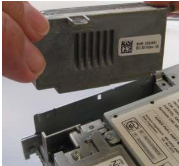
Figure 12. Insert the new telephone module.
