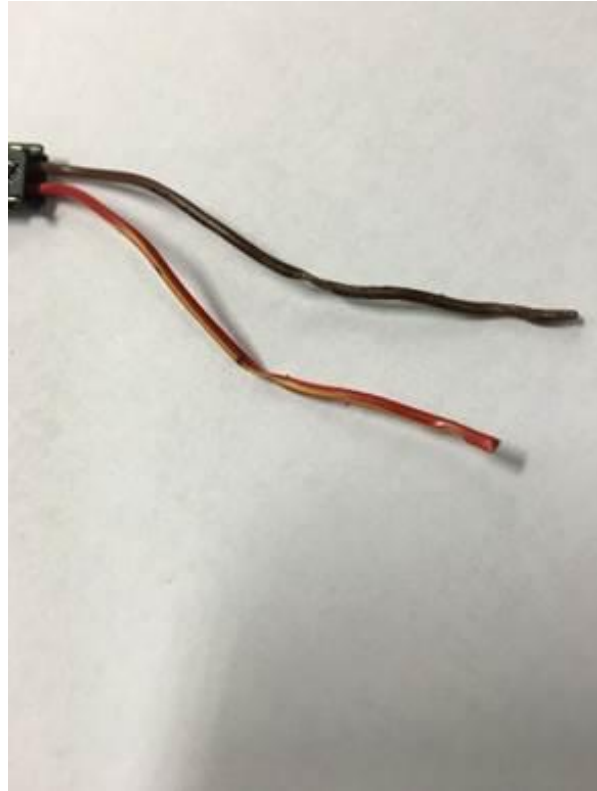
Figure 5. Damage typically found on roof harness.
