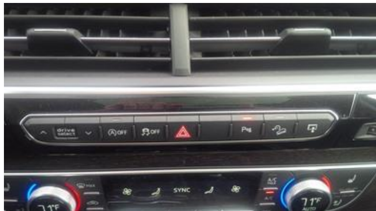
Figure 1. LED on Park Assist button E266.
