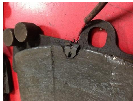
Figure 7. Worn brake pad.
