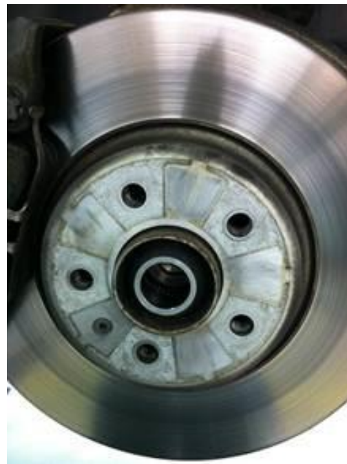
Figure 3: Brake disc with heat marks.
