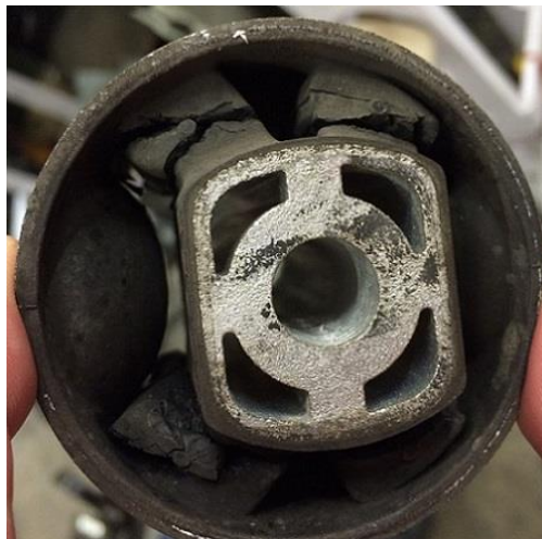
Figure 8. Damaged suspension bushing.
