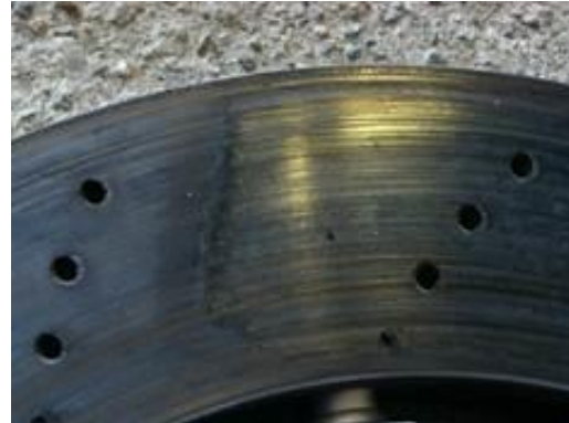
Figure 2. Deposits on the brake disc.
