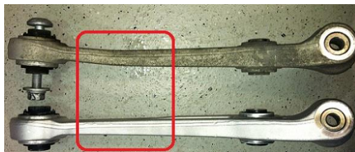
Figure 9. Damaged suspension link.
