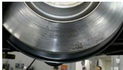
Figure 5. Pad marks on the brake disc.
