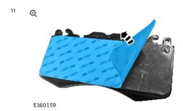
Gently remove the brake pad backing.
