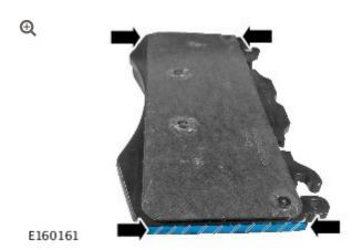
Apply long life lubricating grease to both ends of the brake pads.
