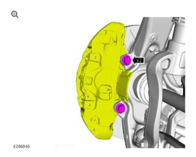
Install the brake caliper.
