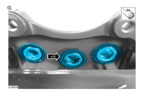
Thoroughly clean all of the brake caliper pistons and the brake caliper piston dust boots with brake cleaner to remove all traces of grease and dust.
