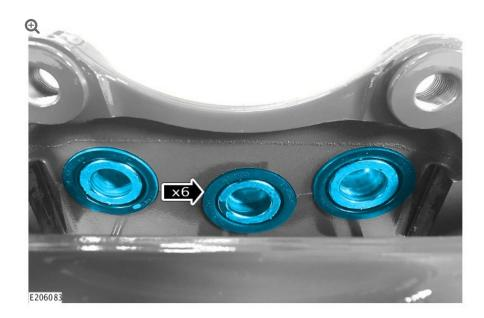
Inspect brake caliper piston dust boots for damage and brake caliper pistons for corrosion.
