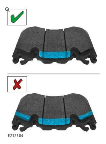
File only the highlighted (✓) center section as shown. Do not file the left and right (X) sections.
