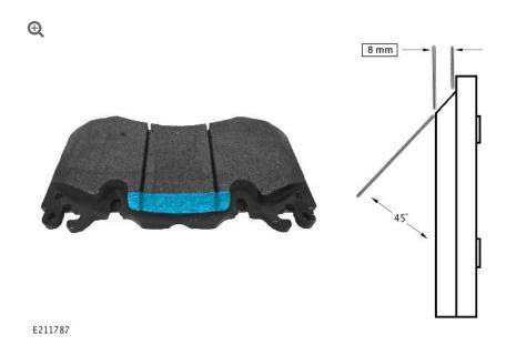
Using a suitable file, file the new front brake pads as shown.
