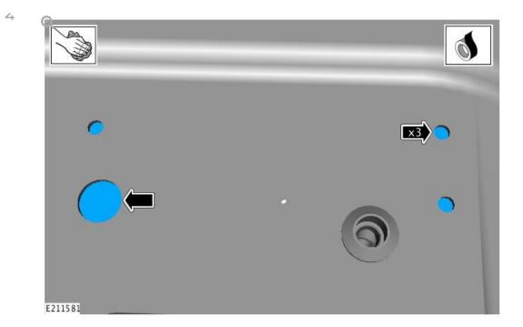
Clean the areas surrounding the 4 holes and install a blanking seal (AZP500060) to each of the 4 holes.
