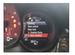
If we have performed coding and communication is lost to the Instrument Cluster; perform a Battery Reset-> deselect the Auto Memory-> Attempt Coding Function. If this does not restore communication, submit a PTEC-> Technical Assistance Request (TLAR).
