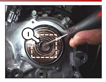
8. Using brake cleaner, spray directly on the motor plug assembly seat (J) inside the motor shaft and clean. Spray brake cleaner on a shop towel to wipe and clean the commutators (K).
