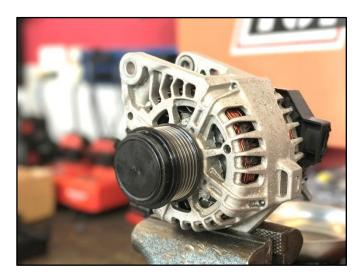
3. Puncture the center of the alternator pulley dust cover (A) with pick and remove the cover.
