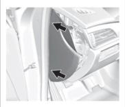
To install the end cover, insert the tabs on the back of the cover into the slots in the instrument panel at the points shown. Align the clips with the slots in the instrument panel, and press the cover into place.
