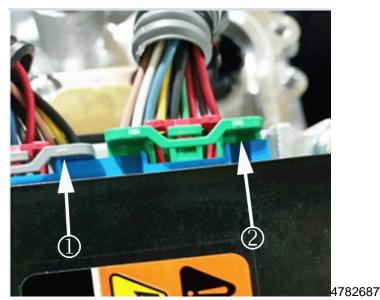
**Note:** The connector position assurance tab (CPA) may be fully engaged, but the connector may NOT be fully seated. In the picture above, the gray connector (1) is fully seated and the green connector (2) is NOT.
