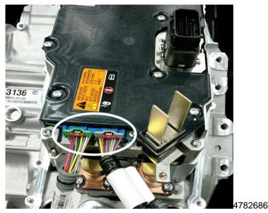
3. Locate the drive motor power inverter module electrical connectors.
