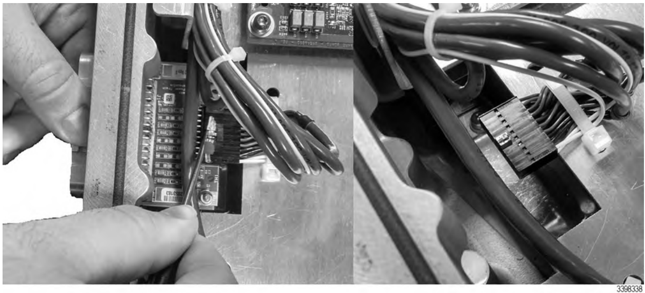
Figure 14. Using Pick to Hold Internal Harness While Removing Encoder Card
