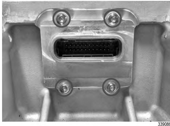
Figure 10. Installing Signal Interface Card Mounting Screws
