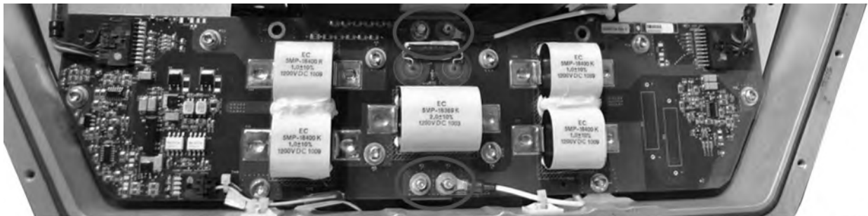
Figure 75. HVIL Circuit Card – Four (4) Mounting Nut/Washer Locations (M5)
