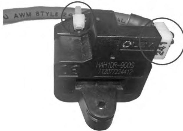
Figure 53. Current Sensor Harness Assembly Wire Tie Location
