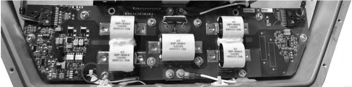
Figure 72. HVIL Circuit Card – Wire Tie Location
