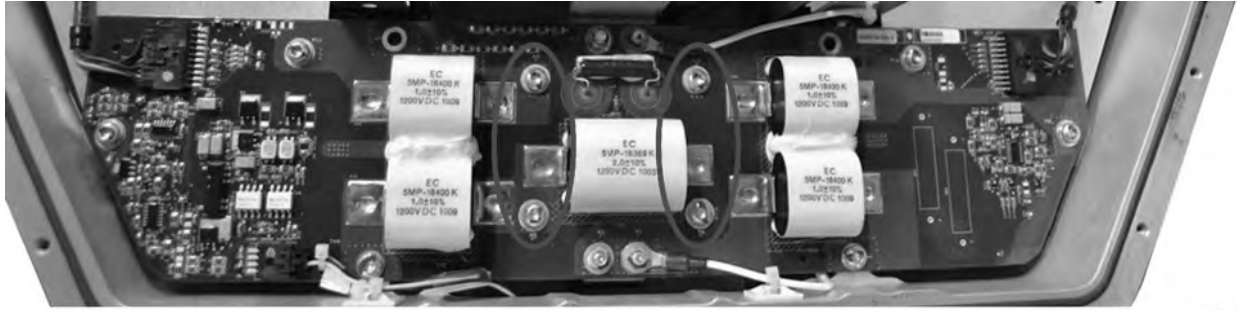
Figure 9. HVIL Circuit Card – Four (4) Mounting Screw Locations (M5x30mm)
