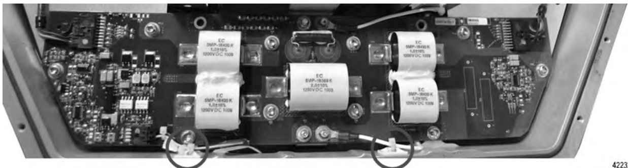
Figure 76. HVIL Circuit Card – Two (2) Wire Tie Locations
