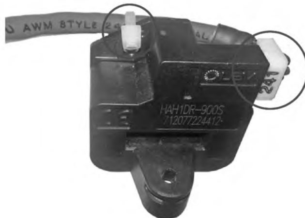
Figure 36. Current Sensor Harness Assembly Wire Tie Location
