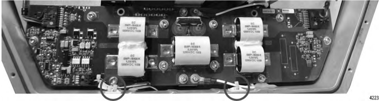
Figure 5. HVIL Circuit Card – Two (2) Wire Tie Locations
