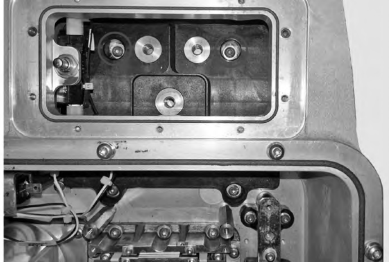
Figure 25. Location of Two (2) M5x22mm Screws
