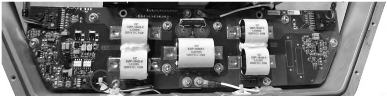
Figure 4. HVIL Circuit Card – Wire Tie Location
