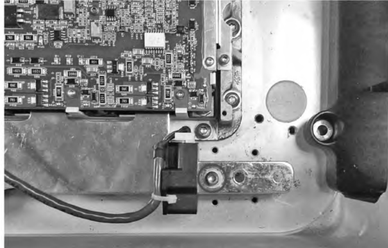
Figure 39. Location of One (1) M4x19mm Screw
