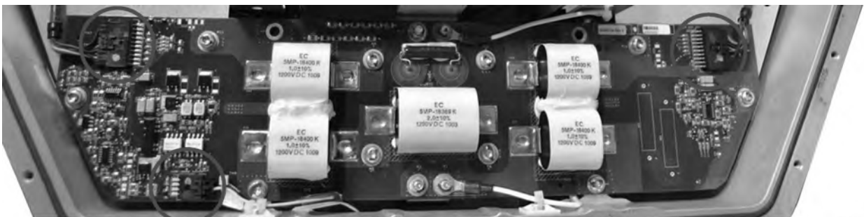
Figure 73. HVIL Circuit Card – Three (3) Harness Connector Locations
