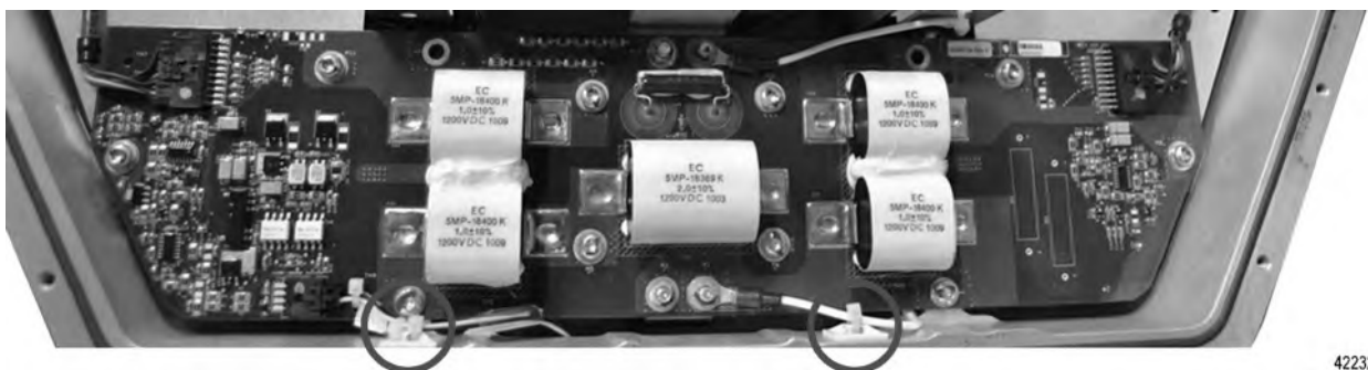
Figure 30. HVIL Circuit Card – Two (2) Wire Tie Locations
