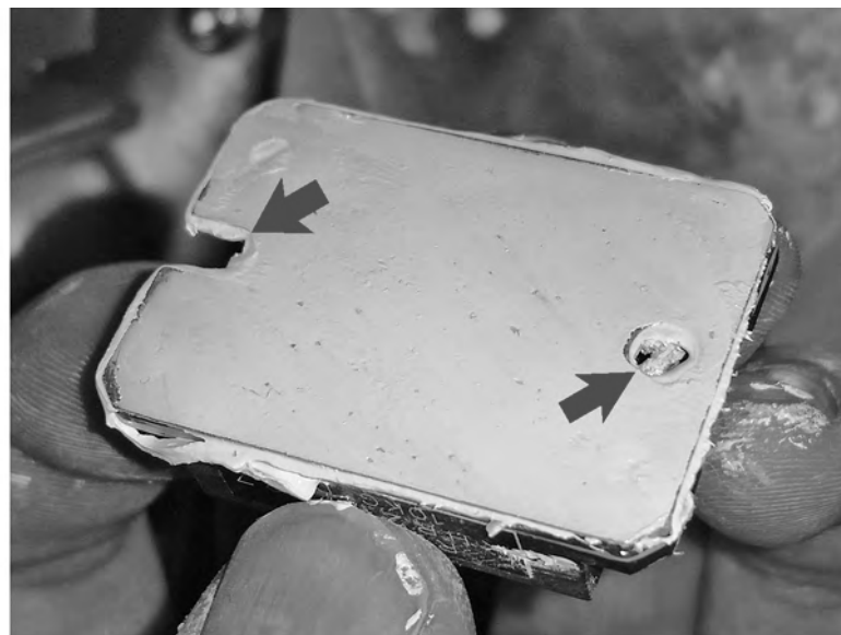
Figure 23. Even Layer of Thermal Compound on Passive Discharge Resistor and Screw Hole Locations
