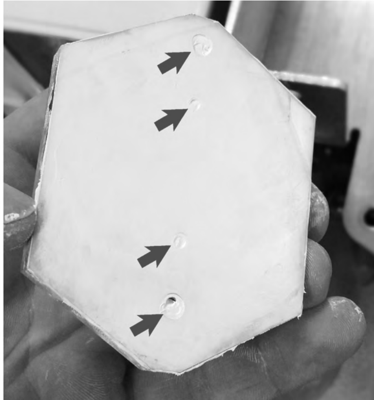
Figure 21. Even Layer of Thermal Paste on Heatsink and Screw Hole Locations
