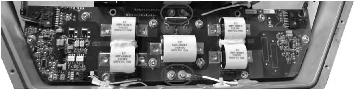
Figure 29. HVIL Circuit Card – Four (4) Mounting Nut/Washer Locations (M5)
