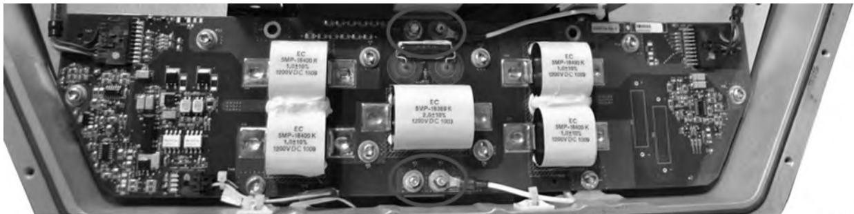
Figure 9. HVIL Circuit Card – Four (4) Mounting Nut/Washer Locations (M5)
