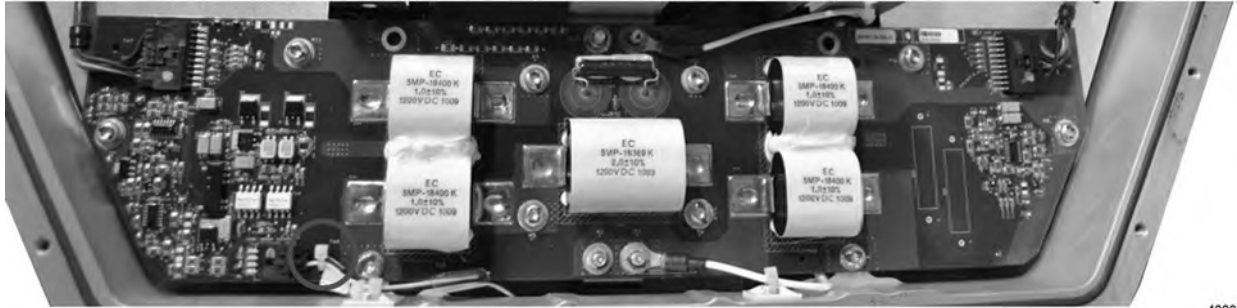
Figure 26. HVIL Circuit Card – Wire Tie Location
