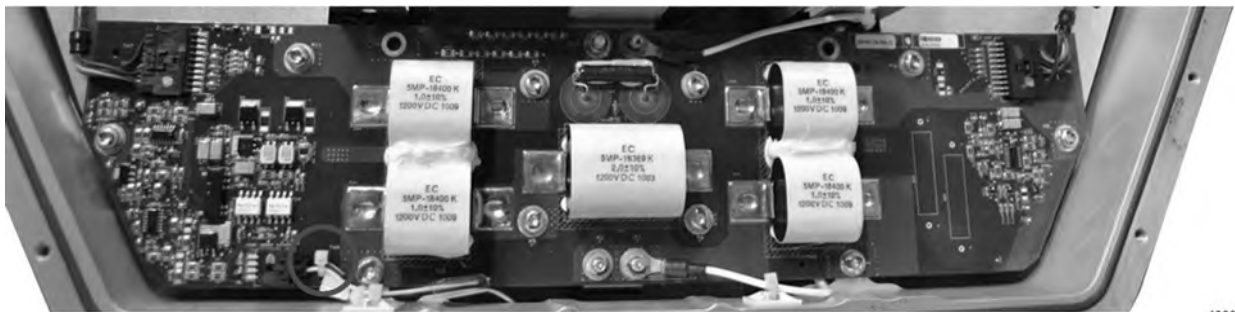
Figure 5. HVIL Circuit Card – Wire Tie Location
