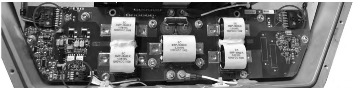
Figure 27. HVIL Circuit Card – Three (3) Harness Connector Locations
