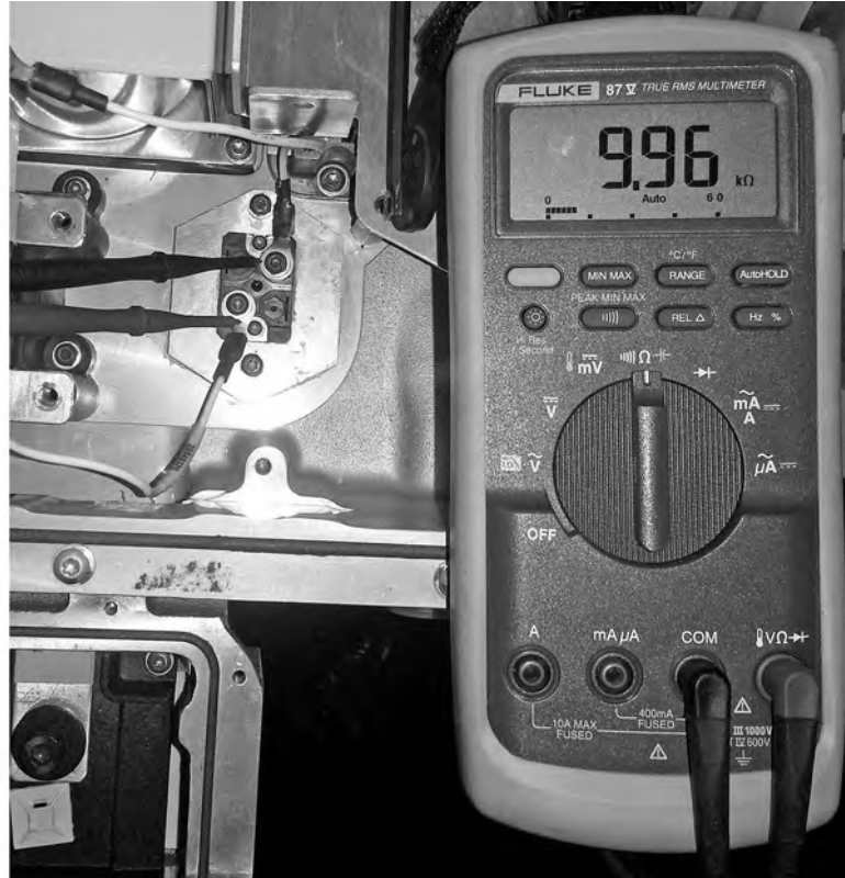
Figure 16. Measuring Resistance Across Passive Discharge Resistor
