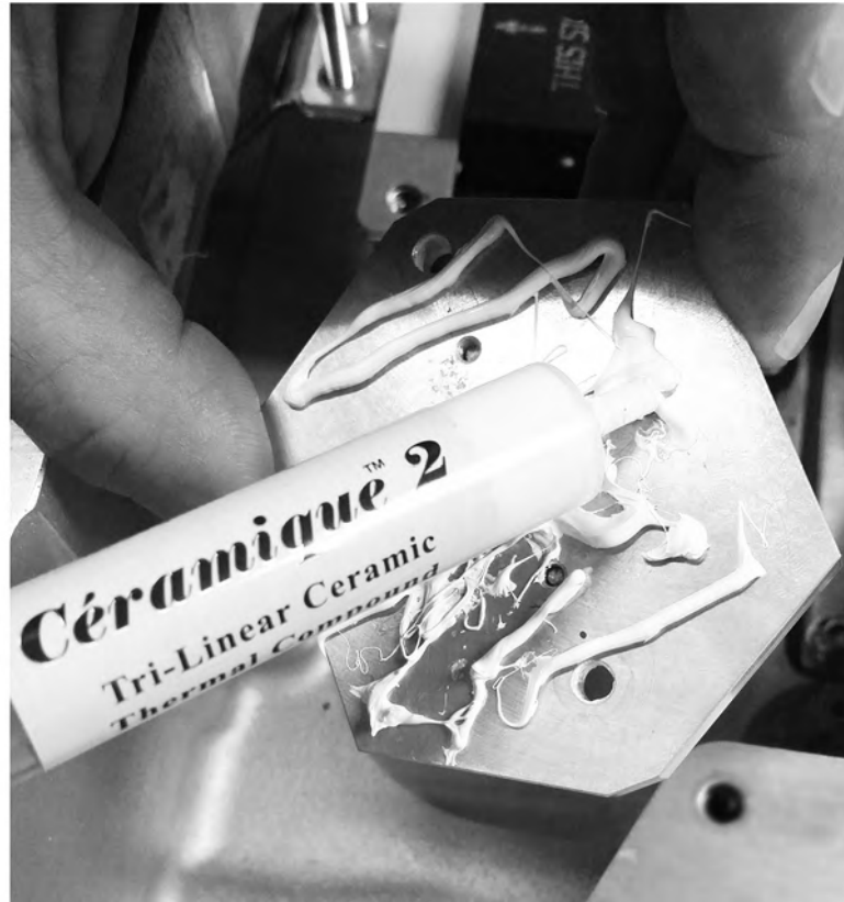
Figure 20. Application of Thermal Compound
