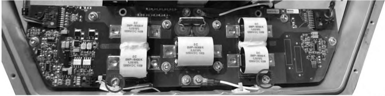
Figure 11. HVIL Circuit Card – Two (2) Mounting Screw Locations (M5 x 14mm)
