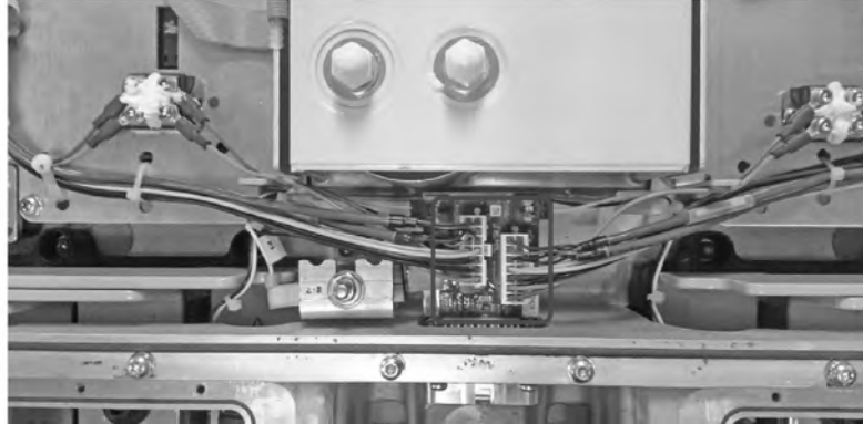
Figure 45. Wire Harness Connector Installation
