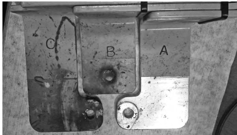
Figure 4. Damage to AC Busbar Caused by Electrical Arcing
