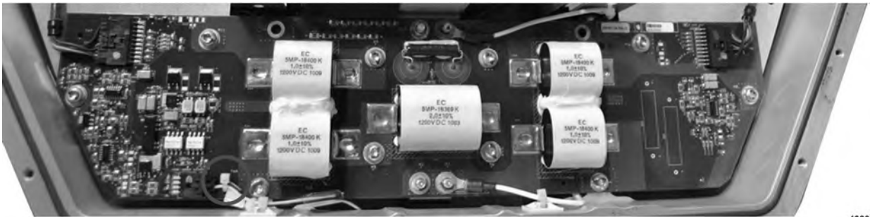
Figure 47. HVIL Circuit Card – Wire Tie Location
