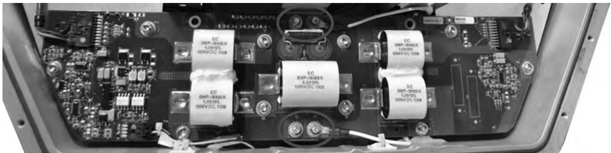
Figure 12. HVIL Circuit Card – Four (4) Mounting Nut/Washer Locations (M5)
