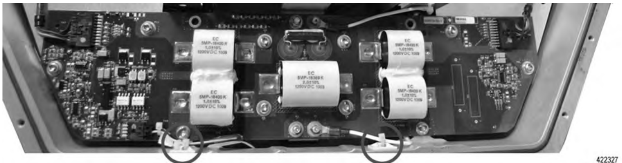
Figure 51. HVIL Circuit Card – Two (2) Wire Tie Locations
