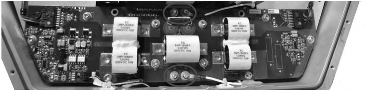
Figure 50. HVIL Circuit Card – Four (4) Mounting Nut/Washer Locations (M5)
