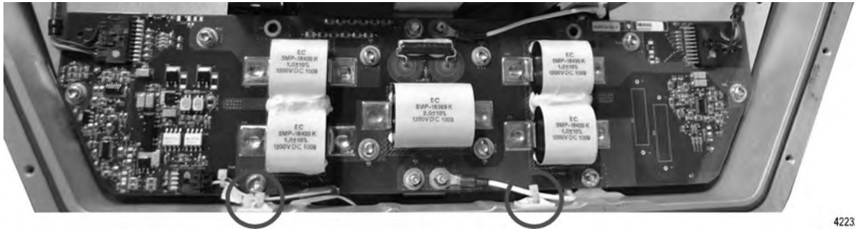
Figure 9. HVIL Circuit Card – Two (2) Wire Tie Locations
