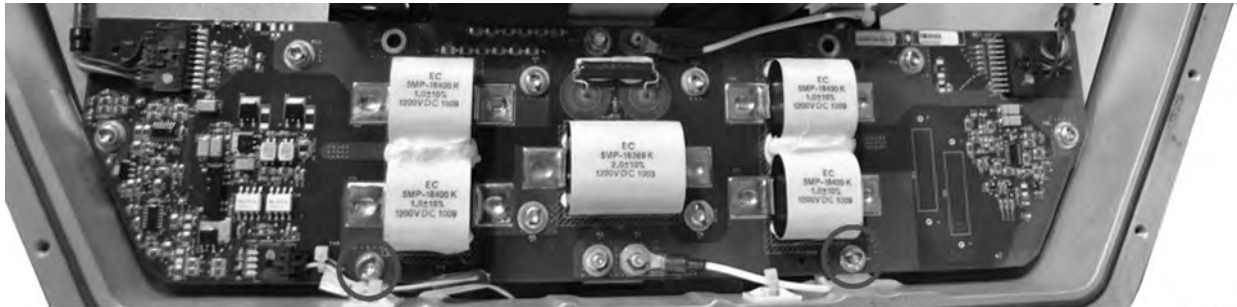
Figure 14. HVIL Circuit Card – Two (2) Mounting Screw Locations (M5x14mm)
