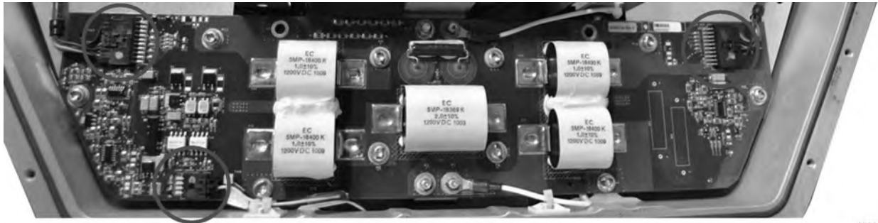
Figure 11. HVIL Circuit Card – Three (3) Harness Connector Locations
