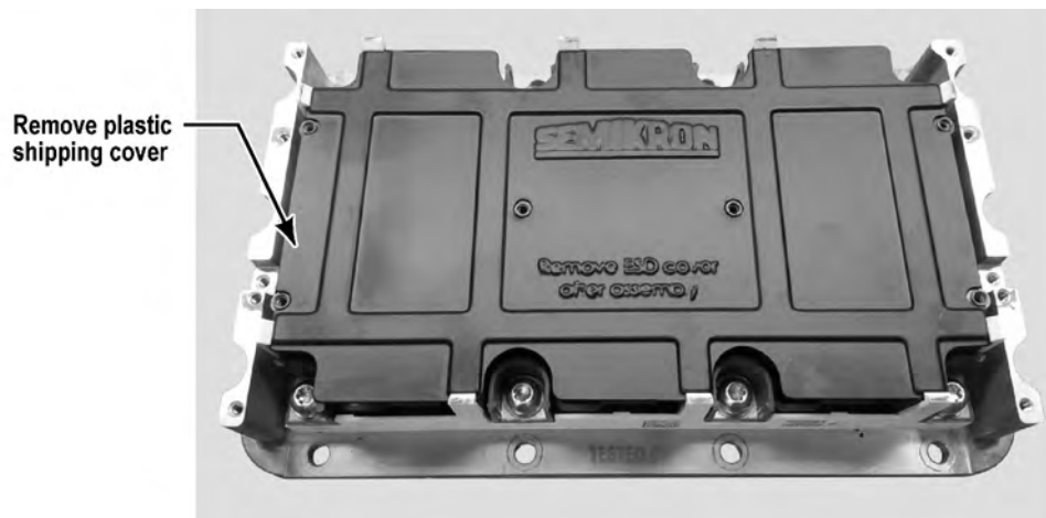
Figure 43. SKiM® Module Plastic Shipping Cover
