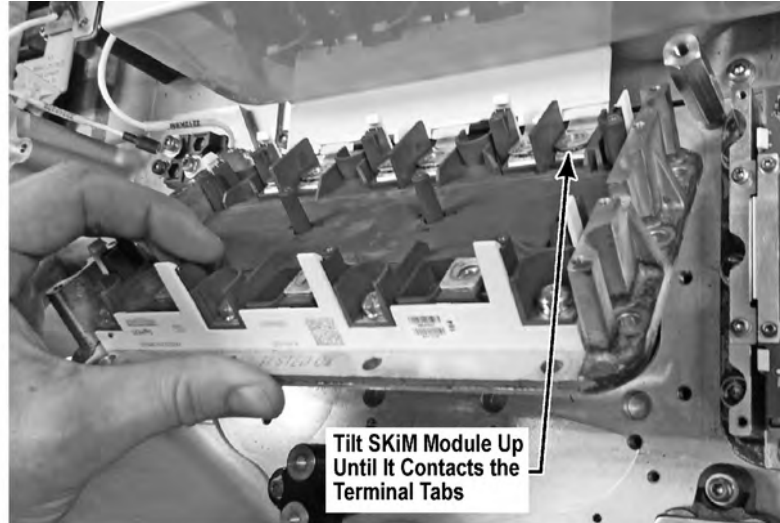
Figure 41. SKiM® Module Removal
