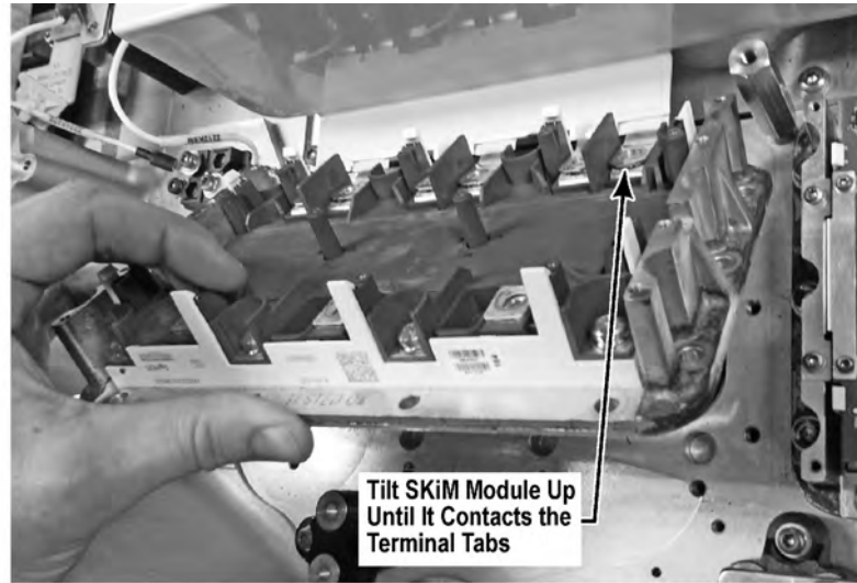
Figure 46. SKiM® Module Installation
