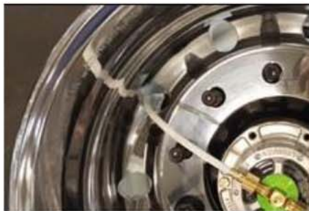
Properly installed tire hose does not touch the wheel
