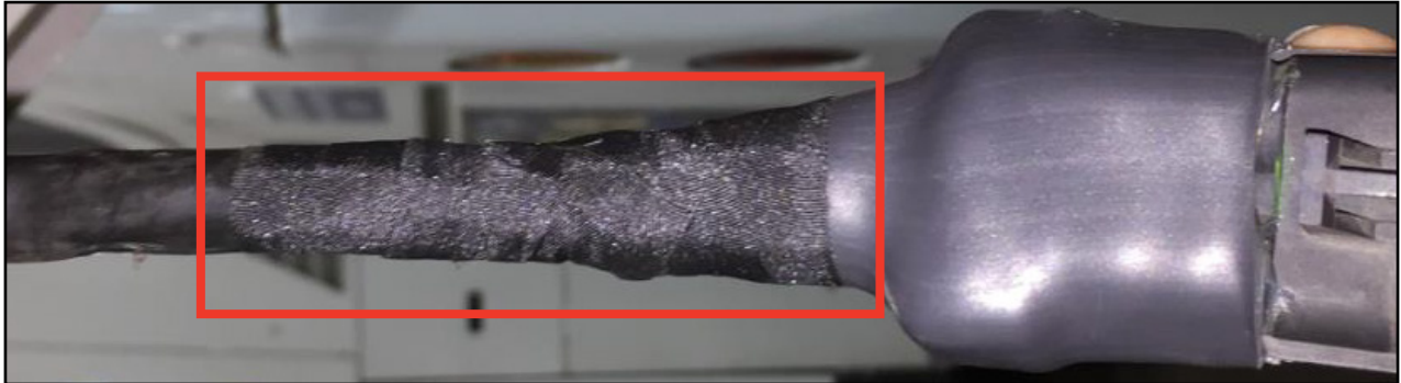
Figure 13 - Typical Installation of Coroplast Tape (N74787)
