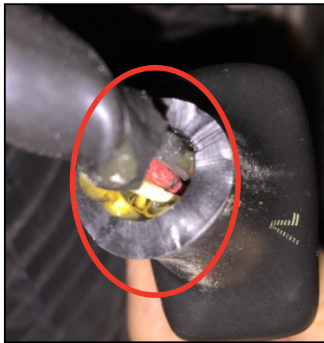
Figure 11 - Tubing NOT Overlapping the Loom
