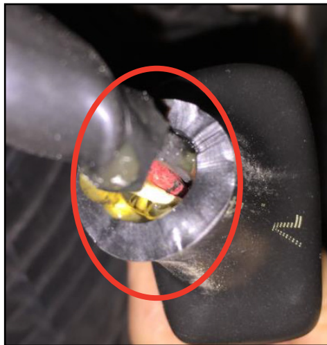
Figure 11 - Tubing NOT Overlapping the Loom
