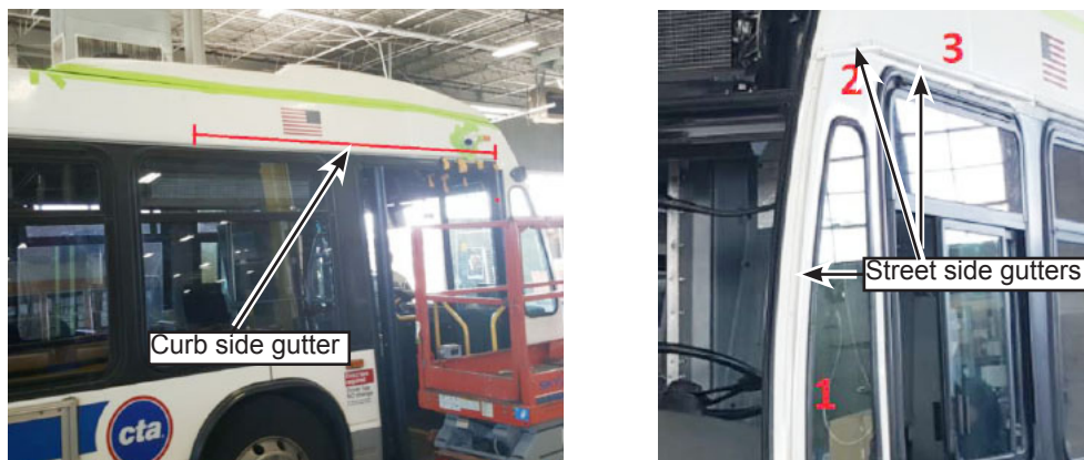
Figure 43 - Install the Gutters
