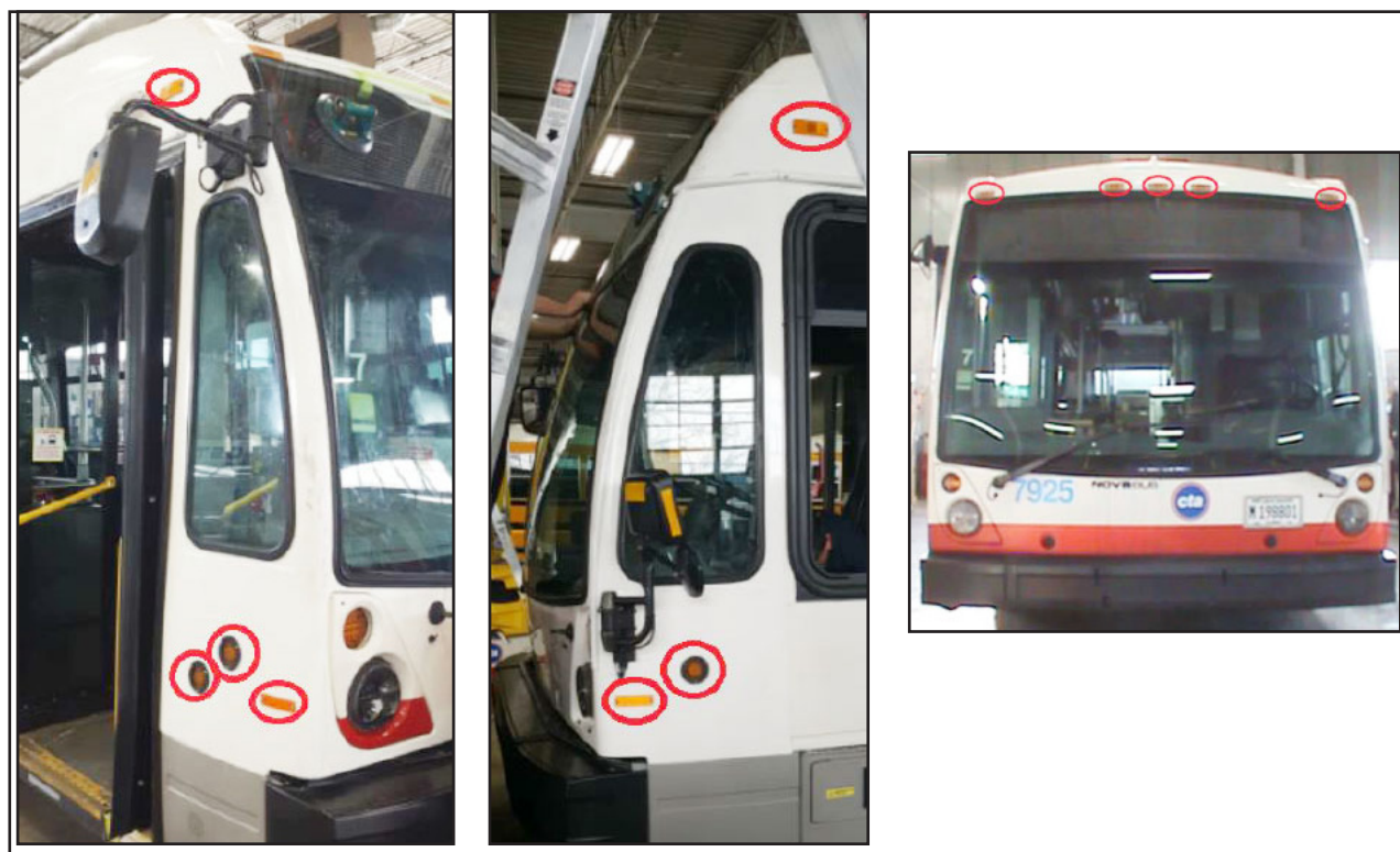
Figure 47 - Install Reflectors, Marker Lights and Signal Lights
