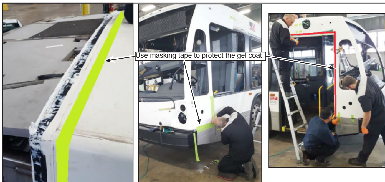
Figure 27 - Protect GelCoat with Masking Tape
