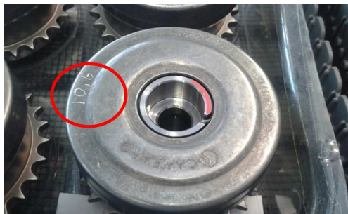
Figure 1 - The stamp previously required on the variable timing mechanisms
