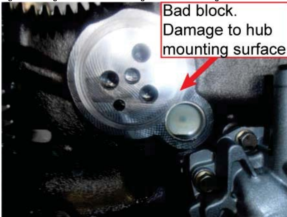
Figure 2 Damaged block. Visible scoring to the hub mounting surface.
