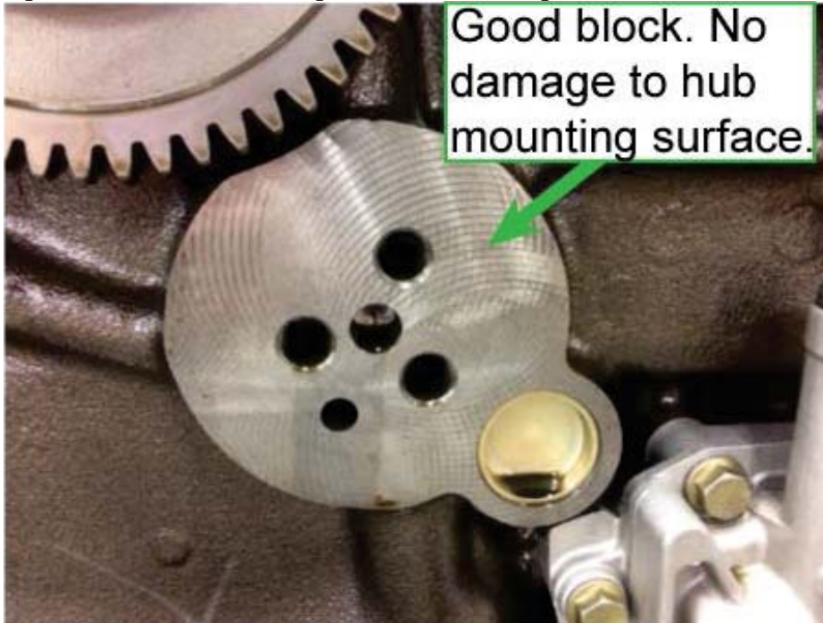
Figure 1 Good block. No damage to the hub mounting surface.
