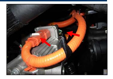
6. Remove 3 bolts and 1 nut. Remove the EOP.
