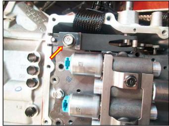
21. Reconnect the solenoid harness to the solenoids and install the temperature sensor.
