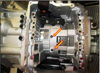
18. Align the manual shaft to the shift lever and install the valve body.
