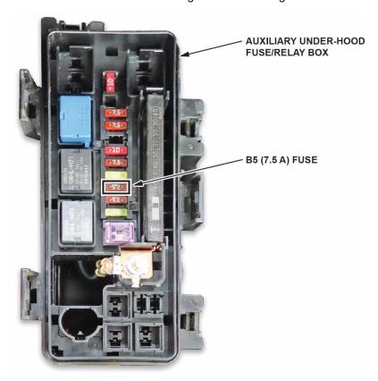
If you get a vehicle in for this issue, check if the brake/taillights and high mount brake light are working when you press the brake pedal. If they aren't, check for a blown B5 (7.5 A) fuse and replace if needed. Then, replace the high mount brake light.
