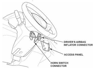
3. Disconnect the driver's airbag inflator connector on the cable reel harness. Disconnect the horn switch connector. Remove the T30 Torx bolts, then remove the driver's airbag module.
