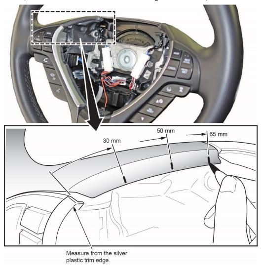
5. Measure 6 mm from the top edge of the spoke down towards the bottom of the leather material, and scribe marks at 30 mm, 50 mm, and 65 mm. Do this on both the right and left side spokes.
