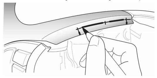
7. Using a new flat razor blade, cut out the rectangle to remove the excess leather material from the steering wheel on both the right and left side spokes.
