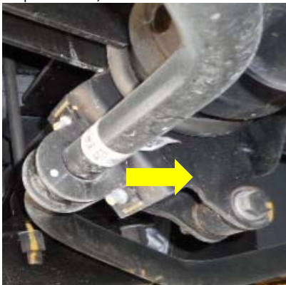
Step 6: Remove/Discard Lower Shock Mount
