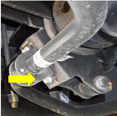
Step 6: Remove/Discard Lower Shock Mount
