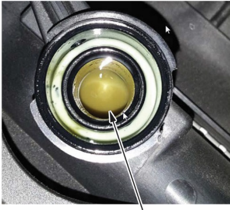
ATF IN THE COOLING SYSTEM
