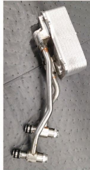
WARMER WITH ACCESSORY COOLER LINES
