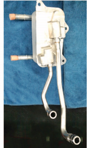
WARMER WITHOUT ACCESSORY COOLER LINES
