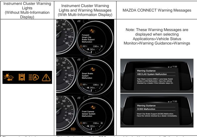
The warning lights/messages will be displayed until the FSC cools and the ignition is turned off, then back on.
