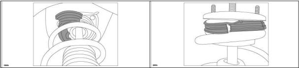
Install Protector onto Coil Spring (For Vehicle Type A, B and E)
