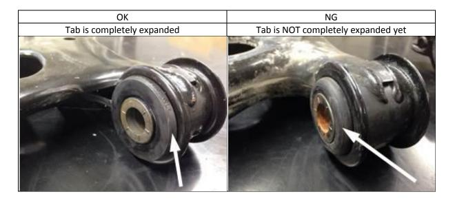
4. After the installation, verify that the front lower arm bushing has been installed to the correct position by the procedure shown in the figure.
