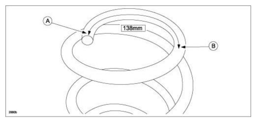
5. Install the protector (A) onto the coil spring aligning the end (slant cut side) with the marking at spot (B).
